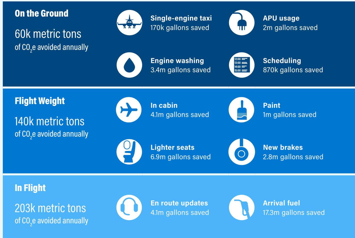
taxi operation (i.e., using just one aircraft engine to taxi to the gate after landing), which reduces the carbon emissions produced by taxiing by 20%–40%. In addition,
